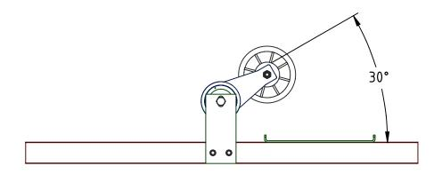
ONCE INSTALLED, PUSH TENSION BRACKET DOWN TO PUT BELT ONTO PULLEY WHEEL
