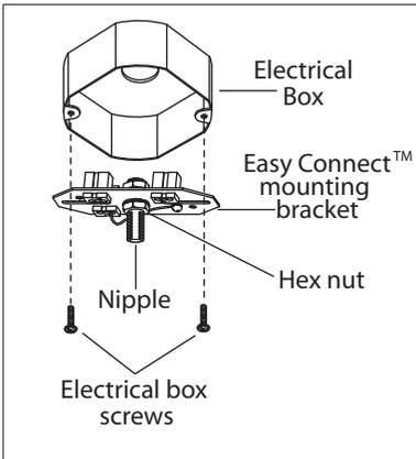
**1.** Attach nipple to mounting bracket. Adjust so it will clear hole in back of fixture and then lock nipple in place with hex nut. Attach mounting bracket to electrical box with electrical box screws (not included).
