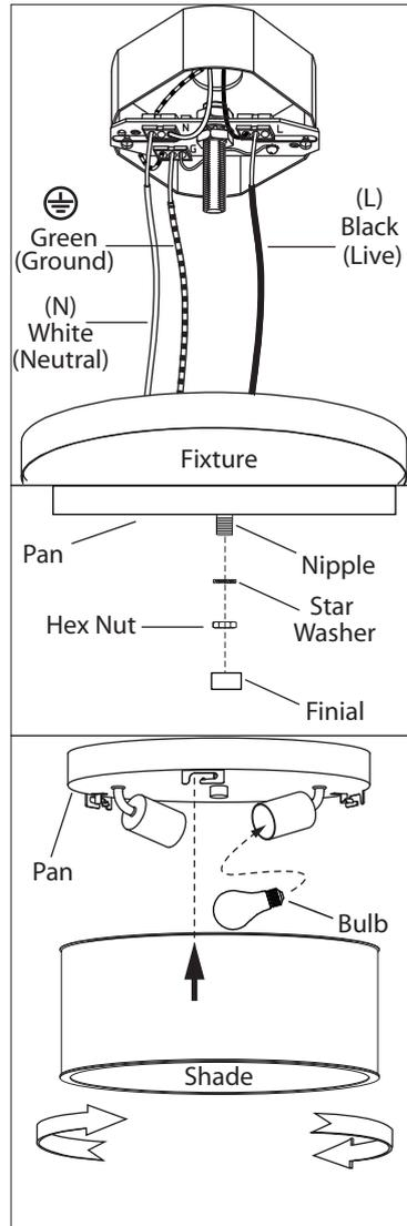
**3.** Connect (push) electrical wires from fixture into correct inserts.
