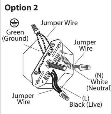
**Option 2:** For multiple green (ground), black (live) and white (neutral) wires joined in the electrical box (house wiring), attach a single "green", "black" and "white" jumper wire before connecting. Strip 7mm from a 6 in. jumper wires supplied. Then connect (push) wires into the correct inserts.
