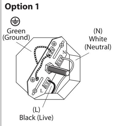
**2. Option 1:** Connect (push) electrical wires from electric box (house wiring) into correct inserts.
