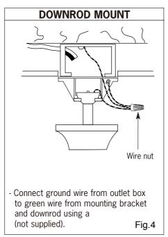
**NOTE**: Once ground wires are connected, carefully tuck wires and wire nut into the outlet box making sure that the wires are clear of the hemisphere and downrod when positioned in mounting bracket (Downrod Mount Only).
