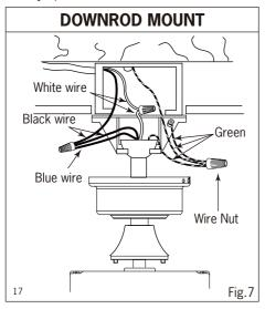
NOTE: Once wires are connected, carefully tuck all wires and wire nuts into the metal outlet box making sure that the wires are clear of the hemisphere and downrod when positioned in mounting bracket (Downrod Mount Only).
