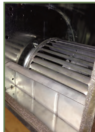
FORWARD CURVED BLOWERS OPERATE AT LOW RPM FOR LOW NOISE
