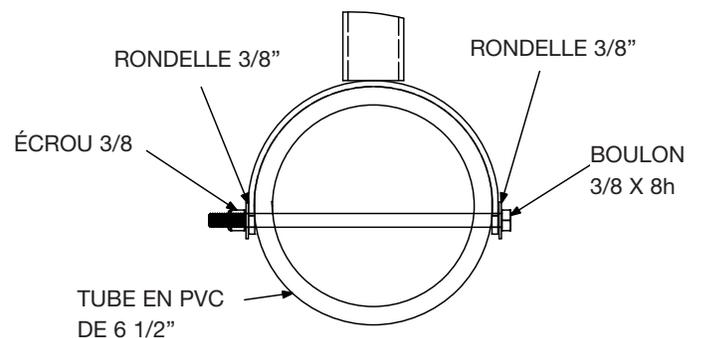
SCHÉMA - LOGETTES MONTÉES SUR COLLET ET MANCHON
