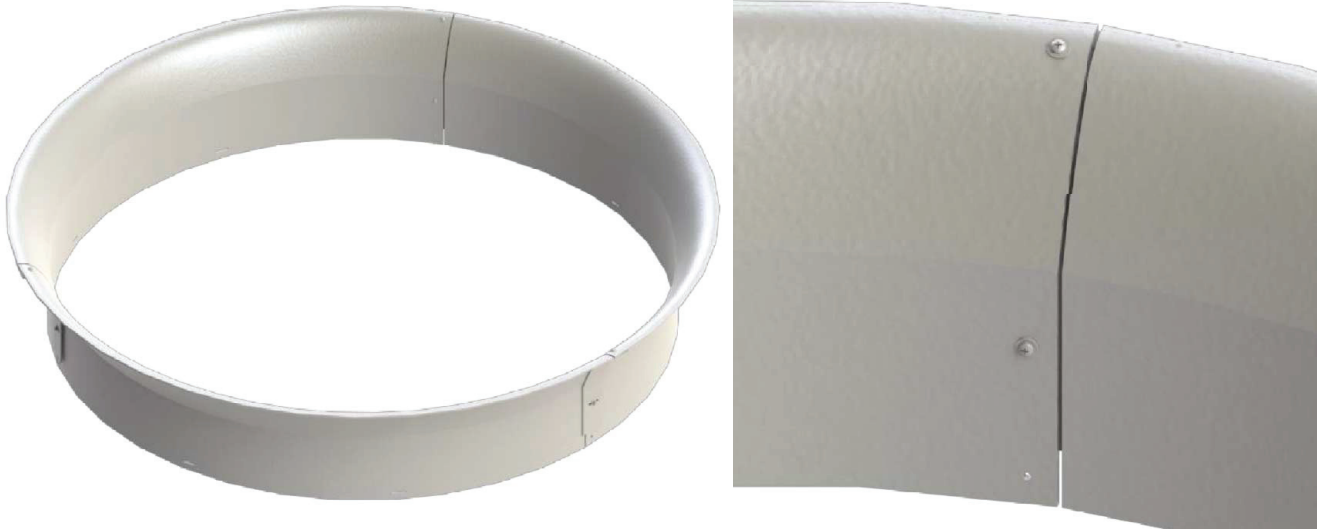
Figure 6 - Installation of the three pieces of the intake together
