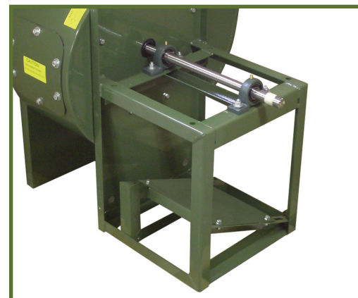
MOTOR AND DRIVE COMPARTMENT WITH COVER REMOVED TO ILLUSTRATE 3 SIDE MOTOR ACCESS AND SLOPED MOTOR BASE FOR BELT TENSIONING.
